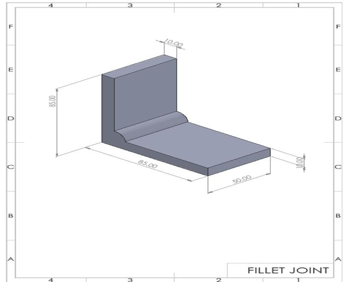
**Figure 1** Graphical illustration of the welded sample joint specimen
