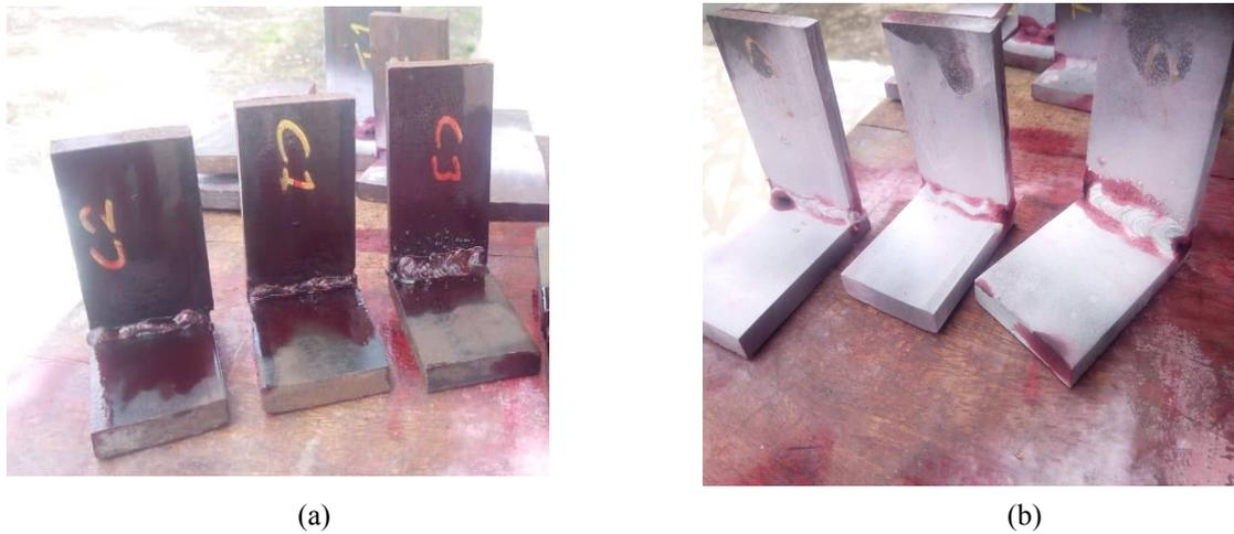
**Figure 5** Sample with (a) dye penetrant applied and (b) results after developer applied
