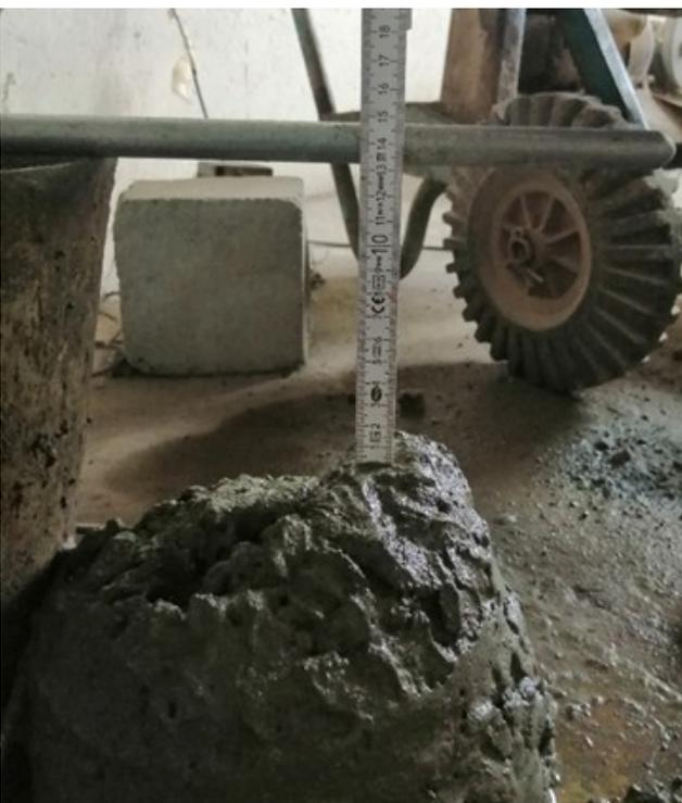
Figure 3 Determination of the slump of concrete
