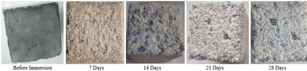
**Figure 13** Visual observation of the SNF concrete specimen at various ages in acidic solution
