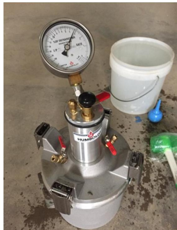
Figure 4 Setup of air content meter
