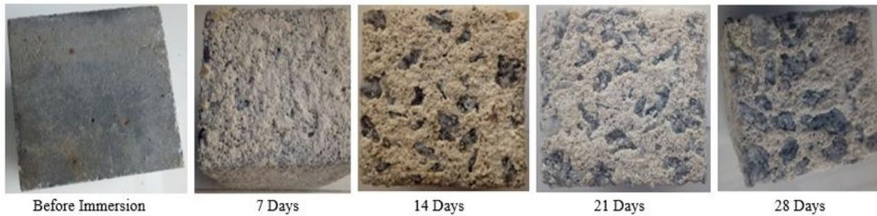
**Figure 12** Visual observation of the control (CON) concrete specimen at various ages in acidic solution
